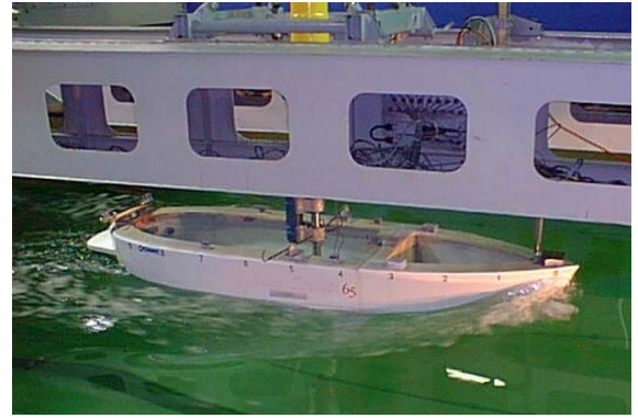
and here's how the competition shapes up.... More wake, more waves — more resistance.
